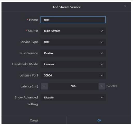
After configuration, click "OK" and the added service will be displayed under the stream service list. The receiving end can pull the stream by copying the full address of the SRT. Or in the Caller mode, fill in the IP and port number (30004) of the aggregation server to pull the stream, the other parameters of the send and receive end are the same.
