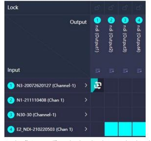
In the "IO Panel", only the display method is different, and the effect of all operations is exactly the same as the "Crosspoint". Click the OUT1 output channel, you can see that the first NDI source is displayed in cyan,
