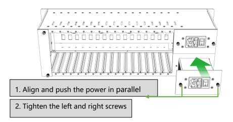
Note: The two power components work uninterrupted at the same time. When one of the components is powered off or damaged, the device will not be powered off. The power components can be replaced without power supply.
