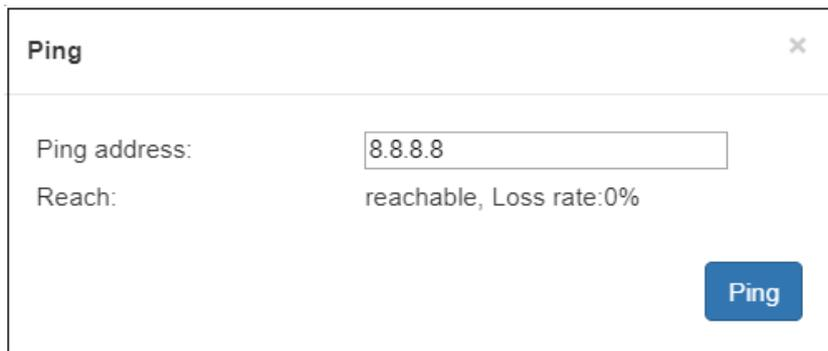
**⚠️ Note:** If Ping public IP address is reachable, but Ping domain name is unreachable. Generally, it is because the DNS server configuration is incorrect.
