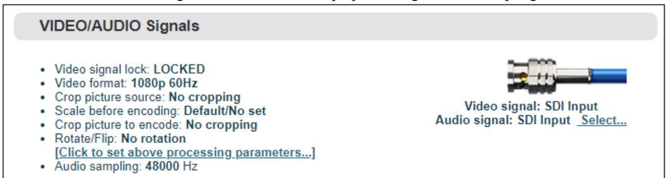
If “video signal lock” displayed as “ no signal (display blue screen)”, it means the video input source is not detected by the device. Please check if the input cable is plugged in. If “Audio sampling” is displayed as “0Hz”, the audio signal is not collected on the device. Please check if the audio of the input source is normal.
