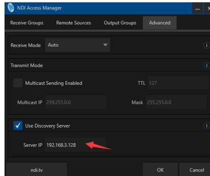
**⚠ Note:** after this function is enabled, the mDNS auto discovery function is invalid. The stream of the decoder can only be sent to the specified server, and the receiver end must register with the same discovery server to pull the NDI stream.
