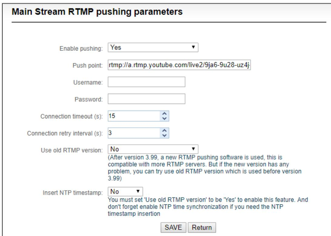
If the platform requires user name and password verification, you also need to fill in the corresponding parameters in the encoder.
