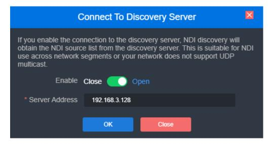
Note: After enabling the discover server, the mDNS auto-discovery function is invalid. The output streams from the encoder can only be sent to the designated server, and the receiving end must register to the same discovery server to pull the NDI streams.
