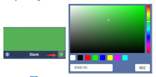
Click the icon on the right to set parameters for smooth switch. To make sure the smooth switch, if it is a big video or slow transmission, a longer smooth time can be set. Otherwise it will show the blank screen set previously when output is not ready after switching.
