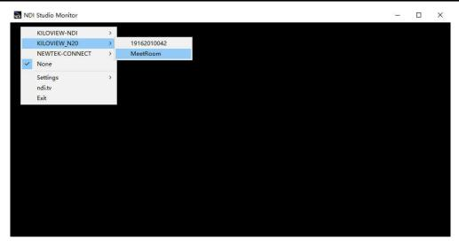
Note: After opening the selected video of the converter by Studio Monitor, click in the lower right corner of the player to open the Web page of the converter directly, which is convenient for the management of the converter.
