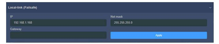
"Failsafe" is to bind the device to an independent IP address. This IP address does not affect the use of other network cards. In special cases, it can be used to manage the encoder. This address can be changed manually (Usually no need to change), the default address is 192.168.1.168.
