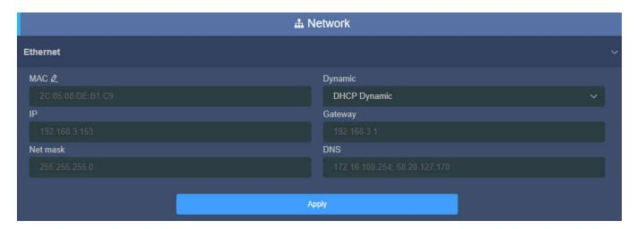
There are two ways to get the address, one is DHCP, and the other is manual setting. To use DHCP to automatically obtain IP, you must first ensure that the router or switch has
