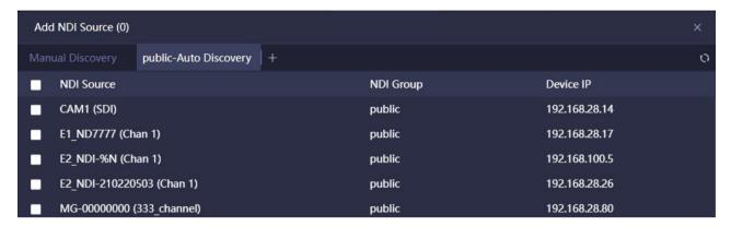
② When the NDI source is in a different NDI group under the same network segment, click <sup>+</sup> to enter the source configuration, and select "Auto ". It will automatically discover all the NDI sources of the current group after entering the name of the group.
