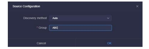
When the NDI source cannot be automatically discovered, such as the NDI source is in the same LAN but across network segments, the NDI source can be added manually by adding IP.
