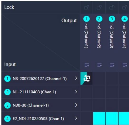
In the "IO Panel", except for the display, all the other operations are exactly the same as "Cross Point". Click the OUT1, you can see that the first NDI source is displayed in cyan, indicating that the NDI video source is output from OUT1, when click the second video source, and it turns cyan, it means that the second one is output from OUT1.
