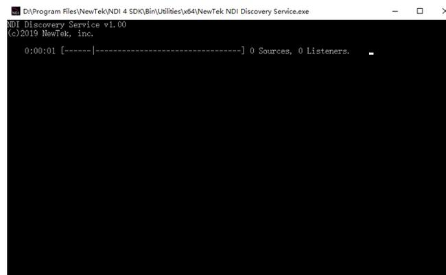
NDI encoder configures the receiving IP address in the discovery server, and NDI will be registered with the server. It is recommended that the receiving address should be configured as a static IP address to prevent the loss of NDI connection due to IP reallocation
