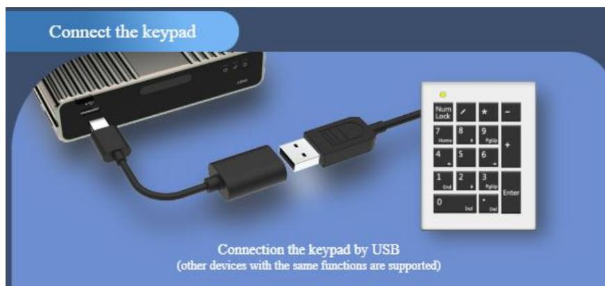
Press **【NumLock】** on the keypad, if the light is on, you can operate the decoding switch. Press 1~9 to select the corresponding 1~9 preset decoding source, and press 0 to select blank
