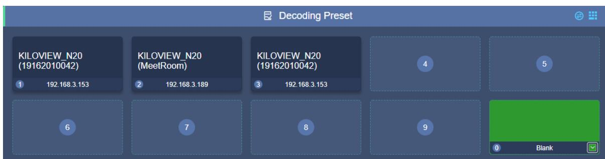
There is a blank output box in decoding preset, if switching to a source without video output, the device will output the set color. It can also be used for testing the output to the monitor by choosing different color.
